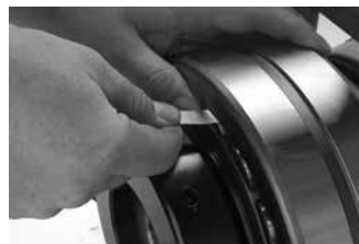
Measure RIC before installation.
